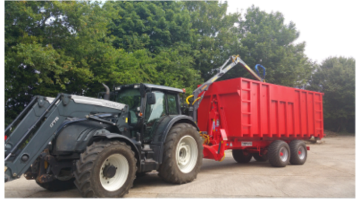
The Hook-lift containers allow the client to easily transport the wood chip using their on-site plant.
