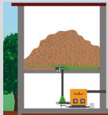
Overhead discharger for woodchip storage.
