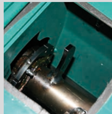
Discharger head with rip hook.
