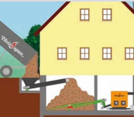
Inclined storage auger for internal fuel storage.
