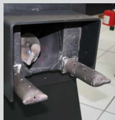
Stoker with primary air ducts.
