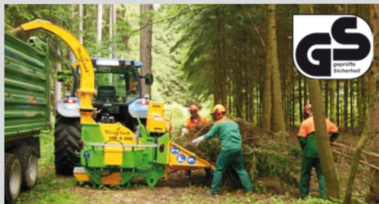
Heizohack hand-feed chipper for 30-40 cm diameter trunk.
