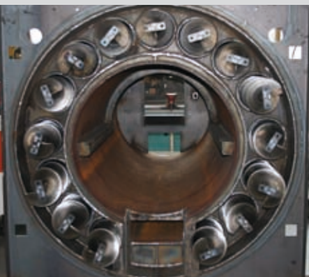
Generous heat exchanger with cleaning auger.
