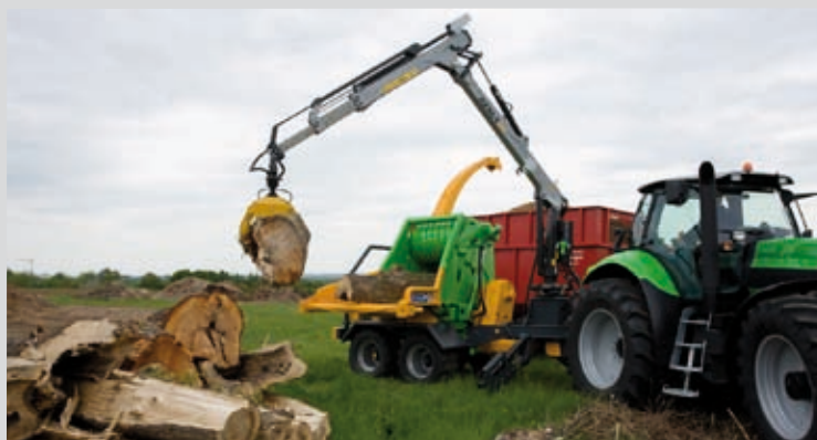
Heizohack crane-feed chipper for 50-80 cm diameter trunk.
