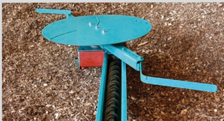
Robust agitator from 1-7 m, for the reliable transportation of fuel.
